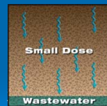
allowing the wastewater to infiltrate into the soil before the next dose is applied
