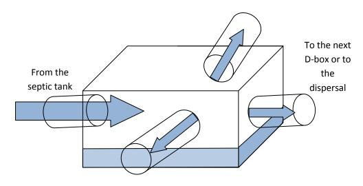
A distribution box can be made of concrete or plastic. It should be installed on a solid base and be extended to within a short distance of the ground surface (or an inspection pipe should be installed).
